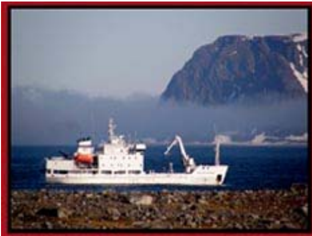
Pic 1: Alexey Maryshev in Bockfjorden – Ship Facts; built in Finland in 1990 and was used by the Russian Academy of Sciences. Contracted by Oceanwide Expeditions. Length: 66 meters, draft: 3.5 meters, top cruising speed: 12.5 knots.
